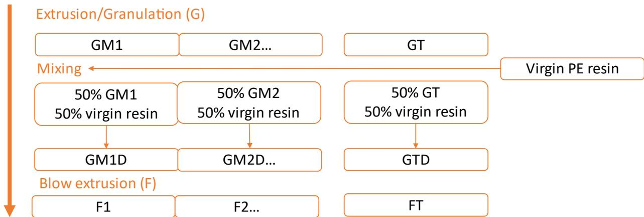
Figure 3: Description of blow extrusion protocol steps
