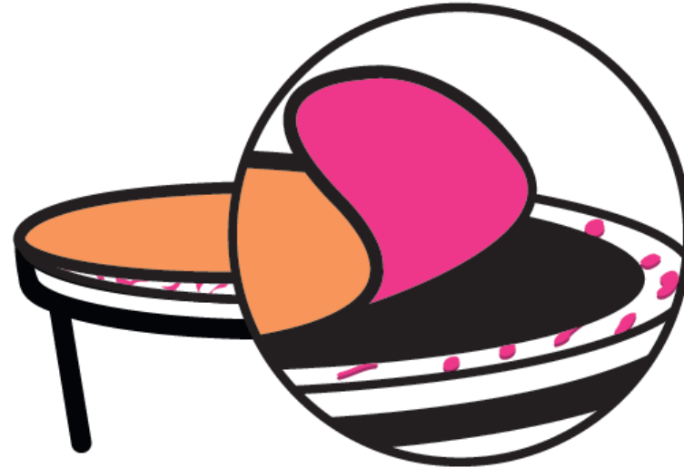
Sealing agent residues on the tray
