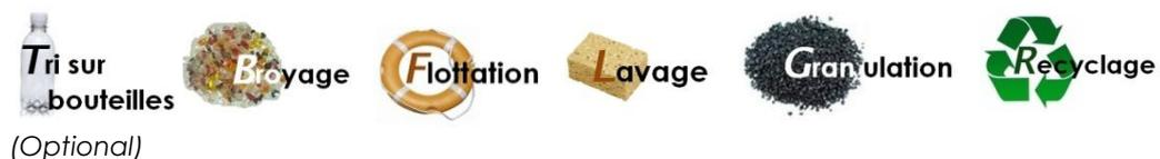
After grinding, the materials are floated in water. With a density of 1 g/cm<sup>3</sup>, water separates the PP flakes from impurities with a density > 1 g/cm<sup>3</sup>. The PP flakes float, and the impurities sink. Only those flakes with a density < 1 g/cm<sup>3</sup> are conserved by the process.
