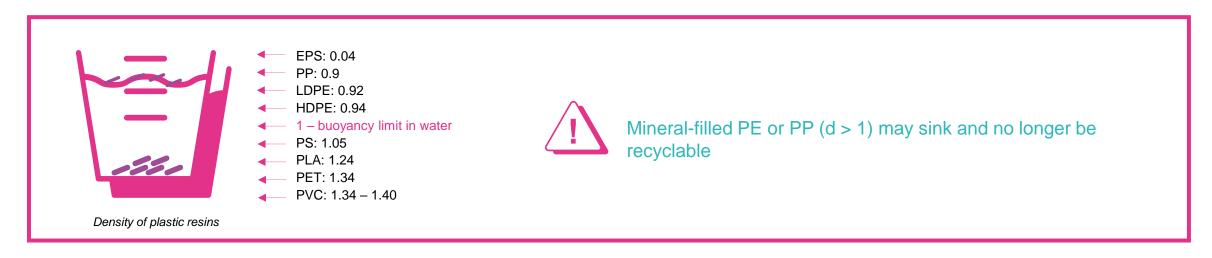
Even if the density does not go over 1, the presence of gases, blowing agents and mineral fillers in the plastic could also have an impact on the mechanical and rheological properties of the recycled material. This impact on the properties of the recycled material has not been evaluated by COTREP to date.
