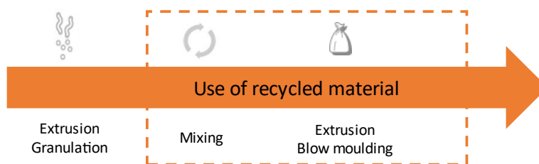
Figure 4: Detailed description of blow extrusion steps
