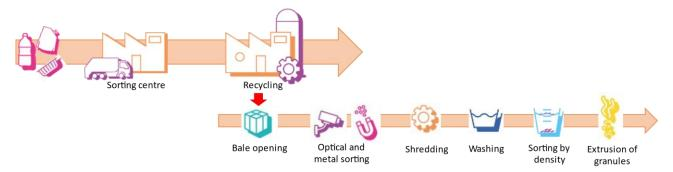
**PET bottles with a partial PE or polyolefin sleeve** are recycled. The majority of sleeves are directed to energy recovery and a small proportion to the cap recycling stream.
