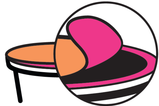
Peelable seal lid Cohesive peelability
