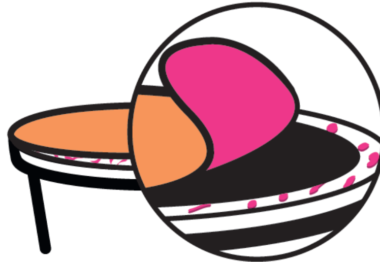
Sealing agent residues on the tray
