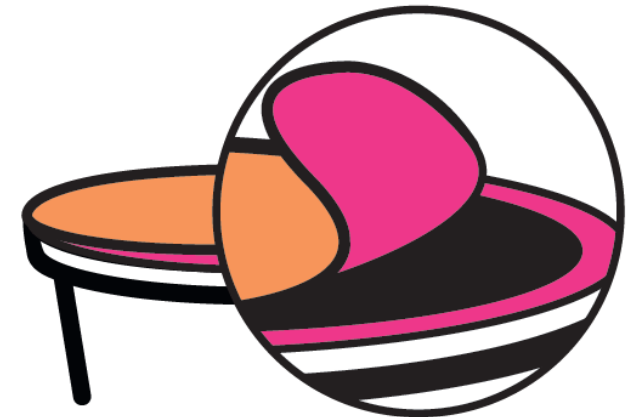
Peelable lid Cohesive peelability
