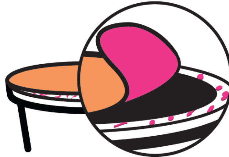
Sealing agent residues on the tray
