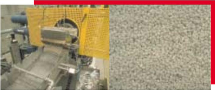
The PET is extruded in wires which are then cut into pellets
